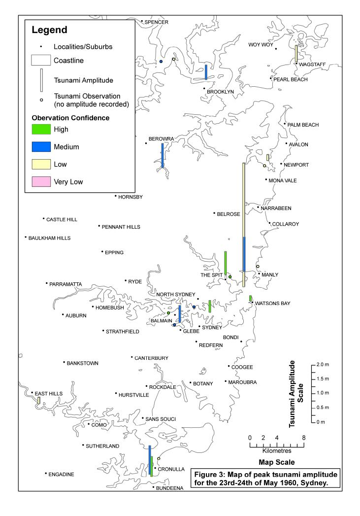
The tsunami did not necessarily dissipate in amplitude as it propagated up these systems. At Bobbin Head, where some moorings were broken, the tsunami amplitude was larger than that observed at other locations on the Hawkesbury River and Broken Bay. At Iron Cove strong currents and damage were reported.
